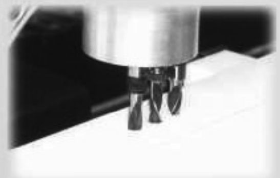
Drills for triple-drill units with male thread or cylindric plain shank
